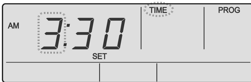
5. Press the **PROG** button to accept the desired hour. Minute field will start blinking.
