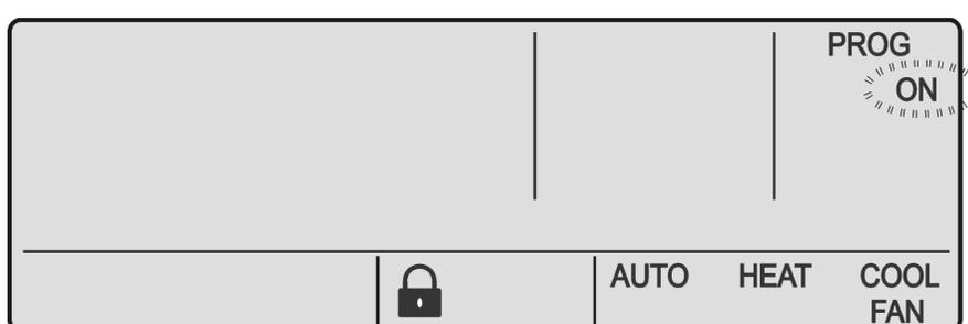
6. Press the **PROG** button to accept the selection. Press the **EXIT** button once to go back to the Main Screen.
