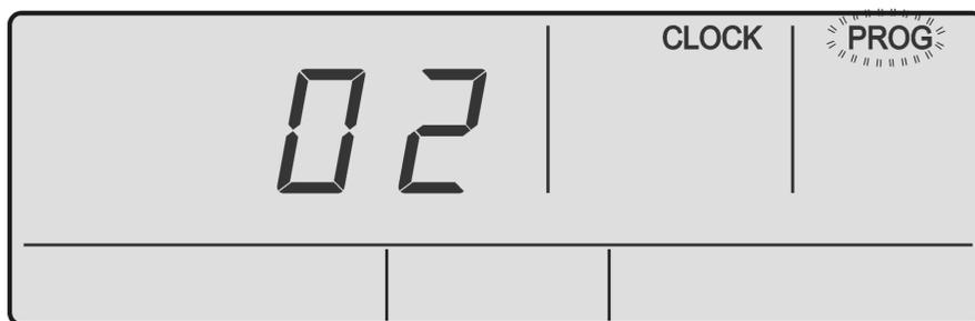
3. Press the **PROG** button to enter Program Menu 02. Display will show clock display. Hour field and **TIME** is blinking.
