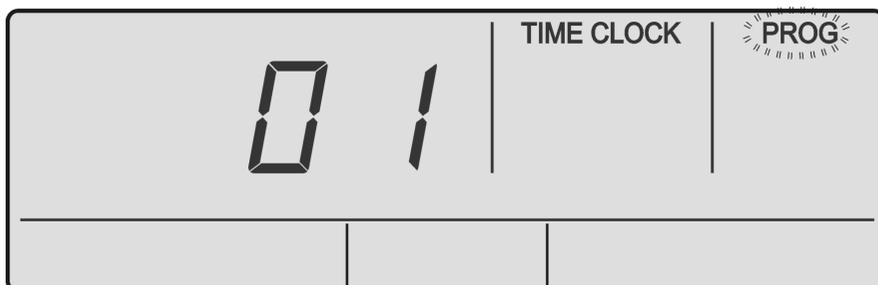
2. Press the **PROG** button to enter the time clock menu. **TIME CLOCK** and **PROG** indicators are still illuminated. **ON** indicator will be flashing in the screen.
