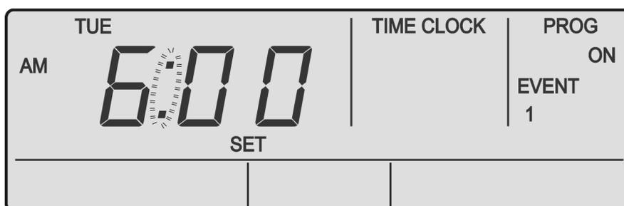
7. Repeat the above steps until you have programmed all the events you require. Otherwise, press the **EXIT** button twice to exit Program Menu. **TIME CLOCK** display will show on the screen to indicate that it is active.
