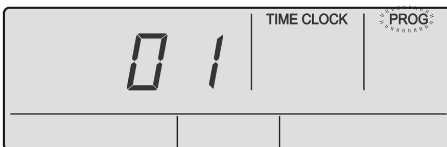
2. Press the **PROG** button to enter the time clock menu. Time clock program is currently On. **TIME CLOCK** and **PROG** indicators are still illuminated. **ON** indicator will be flashing in the screen.
