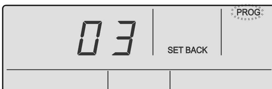
3. Press the **PROG** button to enter Program Menu 03. Display will show set back display **ON** field is blinking.
