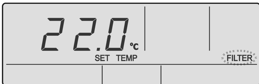
2. After cleaning the filter, press the
