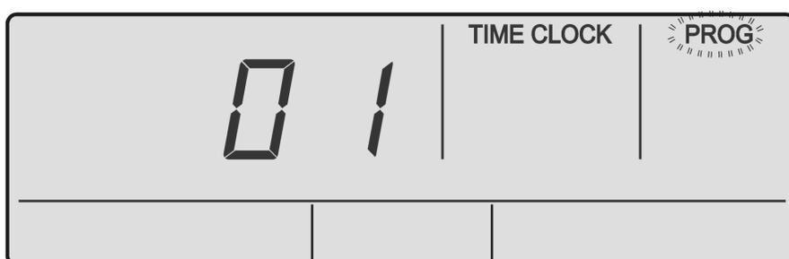
2. Press the **PROG** button to enter the time clock menu. By default, Time clock program is Off. **TIME CLOCK** and **PROG** indicators are still illuminated. **OFF** indicator will be flashing in the screen.
