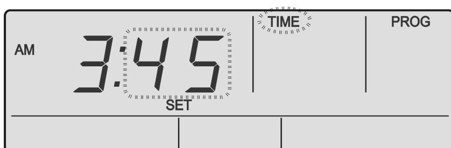
7. Press the **PROG** Button to accept the desired minutes. Day field will start blinking. Day indicator will be flashing, i.e. **MON**.
