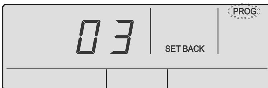
3. Press the **PROG** button to enter Program Menu 03. Display will show **SET BACK** indicator and **OFF** field is blinking.
