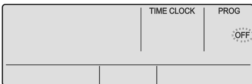
4. Press the **PROG** button to accept the selection and re-activate the time clock.
