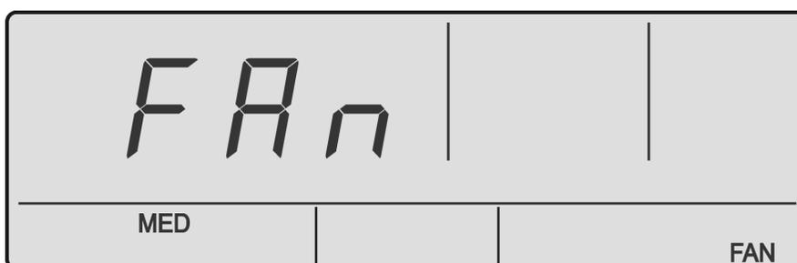
2. Adjust the Indoor Fan speed (**LOW**, **MED** and **HIGH**) by pressing the
