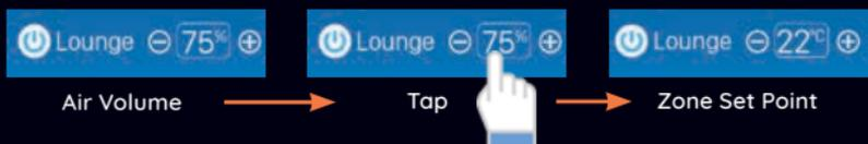
The air volume will automatically adjust according to the difference of set temperature and measured temperature in the zone.
