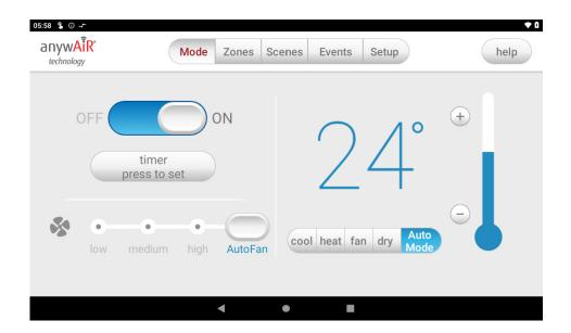
This feature is ideal for ever-changing weather conditions during the day and night. AutoMode will change the mode to heat on a chilly morning and to cool during a hot midday. Like in MainTemp, it will automatically assign the MainZone to an open zone that needs a higher requirement.
