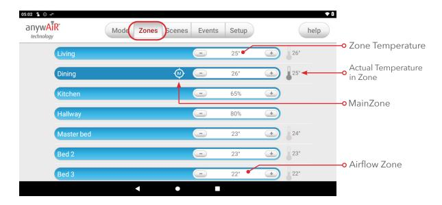
Pressing a Zone name toggles that Zone between ON and OFF. Zones are OFF when they are in grey colour.
