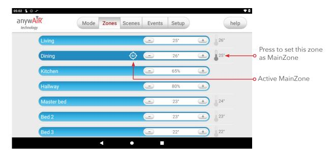
This feature can be particularly important when you have an unusually high requirement for air conditioning in a particular area. For example, a group of people watching a movie in Theatre room with all the electronic A/V equipment turned on will have a larger requirement for air conditioning than in other rooms in the house. Setting the Theatre as MainZone will ensure that the system continues running until the temperature set-point for that room is achieved.
